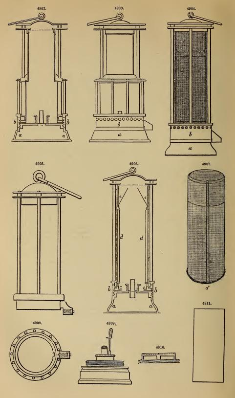
while the glass remains intact. The upper end of this brass tube is closed by a plate of perforated copper brazed to the tube. The outlet is protected in the same manner as in the No. 1.
